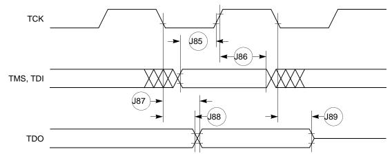
Figure 35. JTAG Test Access Port Timing Diagram
