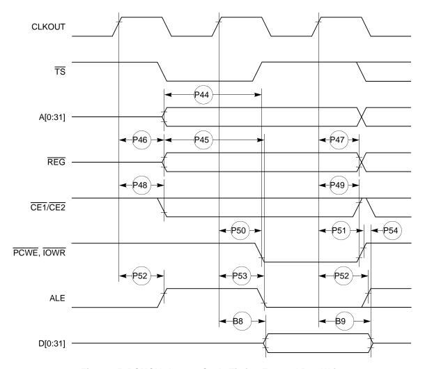
Figure 25. PCMCIA Access Cycle Timing External Bus Write
