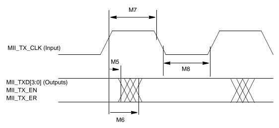
Figure 72. MII Transmit Signal Timing Diagram
