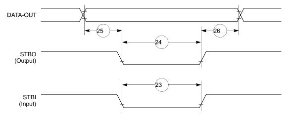
Figure 41. PIP TX (Pulse Mode) Timing Diagram
