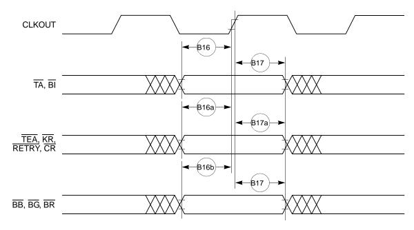
Figure 6. Synchronous Input Signals Timing
