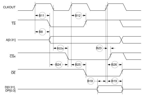
Figure 10. External Bus Read Timing (GPCM Controlled—TRLX = 0, ACS = 10)
