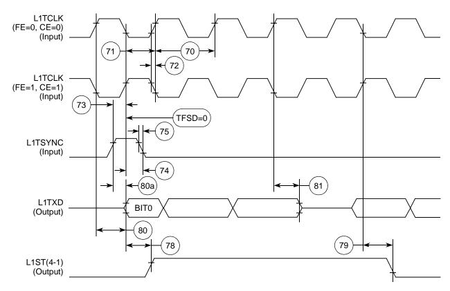
Figure 52. SI Transmit Timing Diagram (DSC = 0)
