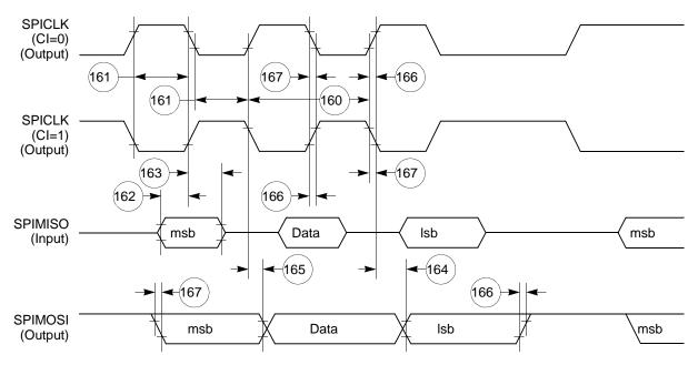
Figure 65. SPI Master (CP = 1) Timing Diagram
