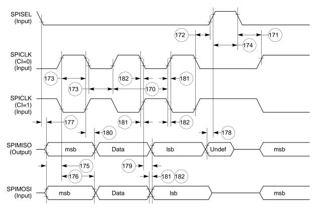
Figure 66. SPI Slave (CP = 0) Timing Diagram
