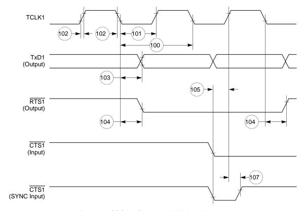
Figure 56. SCC NMSI Transmit Timing Diagram
