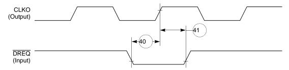
Figure 44. IDMA External Requests Timing Diagram
