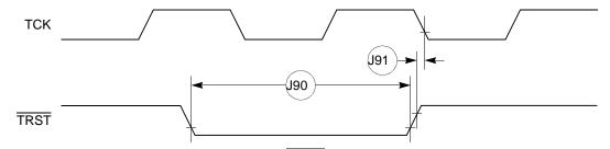
Figure 36. JTAG TRST Timing Diagram
