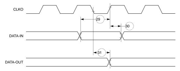
Figure 42. Parallel I/O Data-In/Data-Out Timing Diagram
