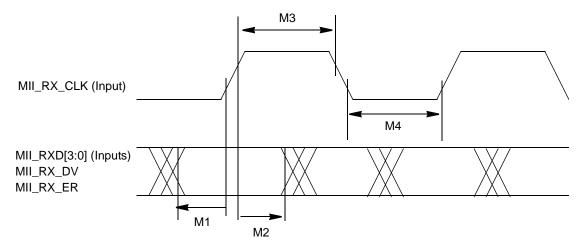
Figure 71. MII Receive Signal Timing Diagram
