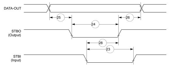
Figure 39. PIP Tx (Interlock Mode) Timing Diagram
