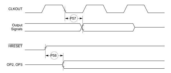
Figure 27. PCMCIA Output Port Timing
