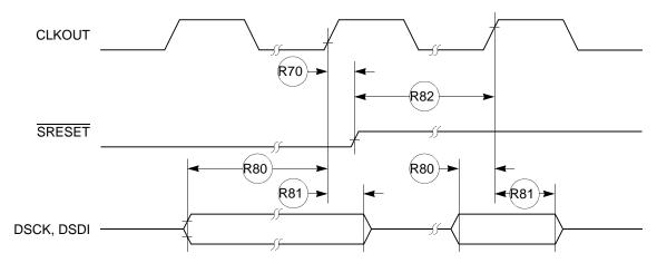
Figure 33. Reset Timing—Debug Port Configuration
