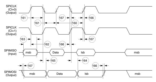
Figure 64. SPI Master (CP = 0) Timing Diagram
