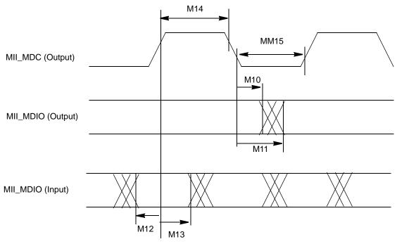
Figure 74. MII Serial Management Channel Timing Diagram
