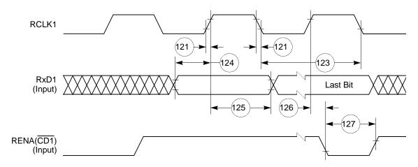
Figure 59. Ethernet Receive Timing Diagram
