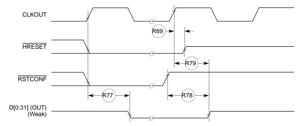
Figure 32. Reset Timing—Data Bus Weak Drive During Configuration
