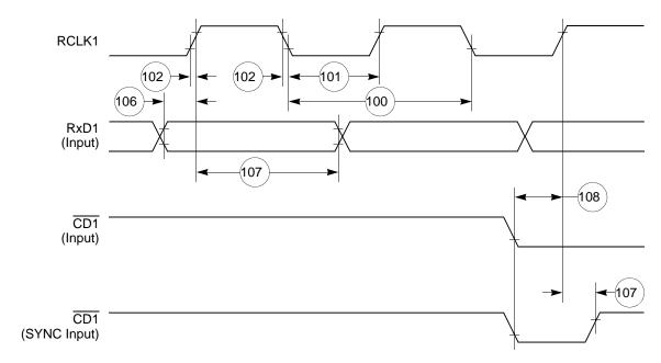
Figure 55. SCC NMSI Receive Timing Diagram
