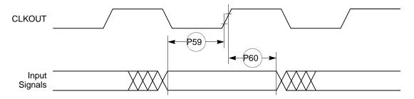
Figure 28. PCMCIA Input Port Timing
