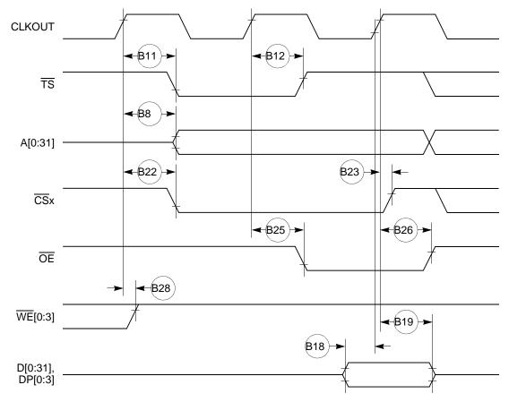
Figure 9. External Bus Read Timing (GPCM Controlled—ACS = 00)
