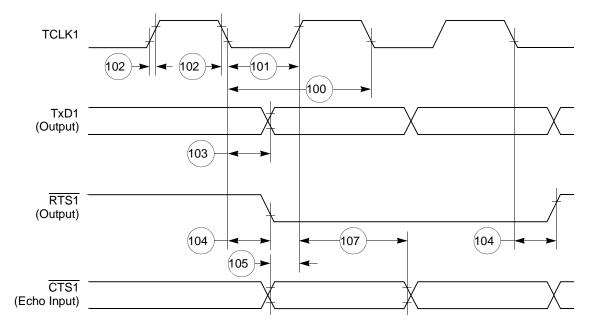
Figure 57. HDLC Bus Timing Diagram
