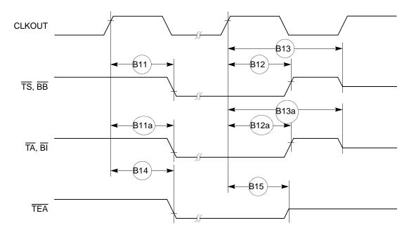
Figure 5. Synchronous Active Pull-Up Resistor and Open-Drain Outputs Signals Timing
