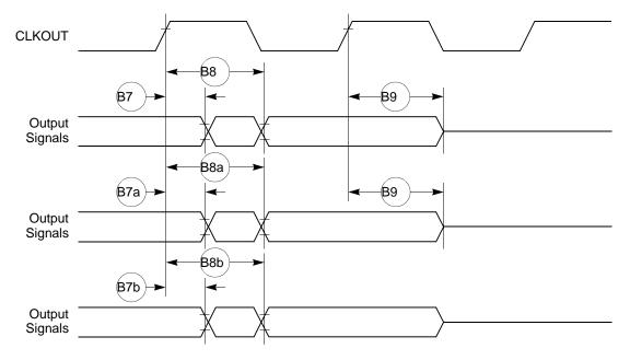
**Figure 4. Synchronous Output Signals Timing**
