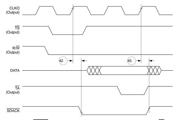
Figure 47. SDACK Timing Diagram—Peripheral Read, Internally-Generated TA
