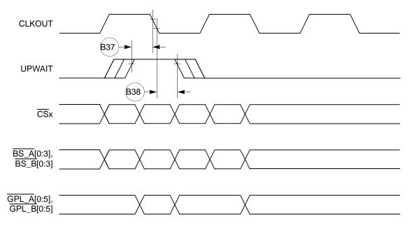
Figure 17. Asynchronous UPWAIT Asserted Detection in UPM Handled Cycles Timing
