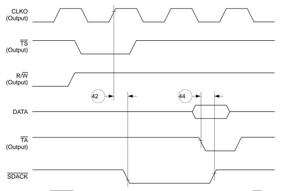
Figure 46. SDACK Timing Diagram—Peripheral Write, Internally-Generated TA
