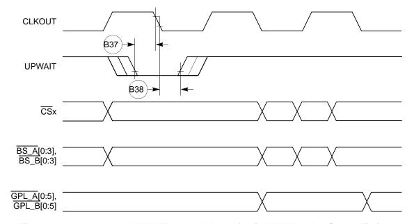
Figure 18. Asynchronous UPWAIT Negated Detection in UPM Handled Cycles Timing
