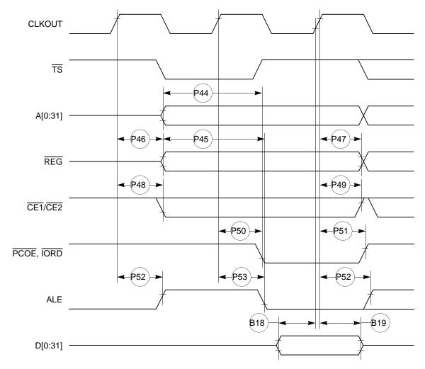
Figure 24. PCMCIA Access Cycle Timing External Bus Read
