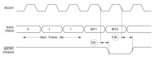
Figure 61. CAM Interface Receive Start Timing Diagram
