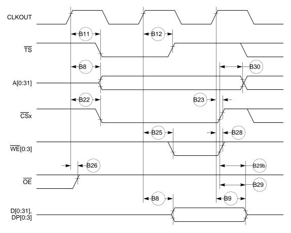
Figure 13. External Bus Write Timing (GPCM Controlled—TRLX = 0 or 1, CSNT = 0)
