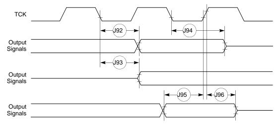
Figure 37. Boundary Scan (JTAG) Timing Diagram
