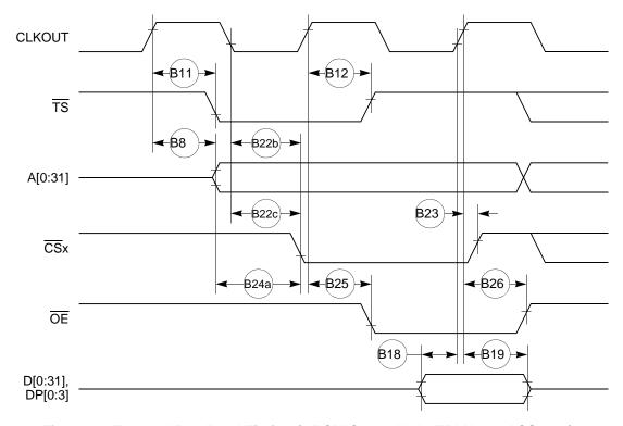
Figure 11. External Bus Read Timing (GPCM Controlled—TRLX = 0, ACS = 11)
