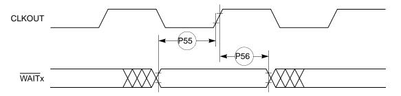
Figure 26. PCMCIA WAIT Signal Detection Timing
