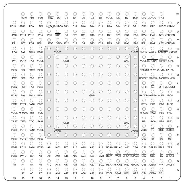
Figure 75. Pinout of the PBGA Package
