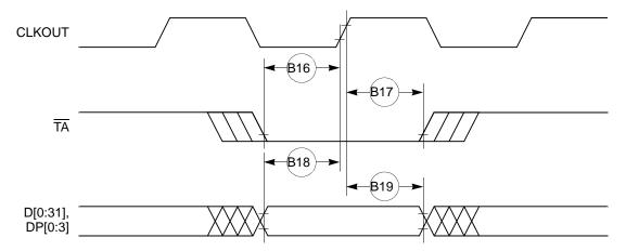
Figure 7. Input Data Timing in Normal Case
