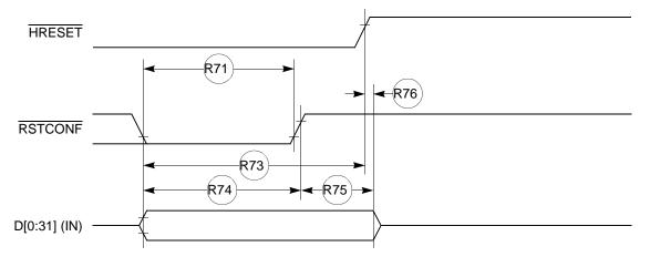
Figure 31. Reset Timing—Configuration from Data Bus
