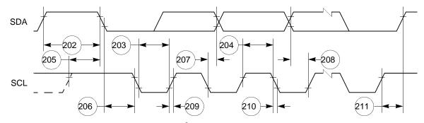
Figure 68. I<sup>2</sup>C Bus Timing Diagram
