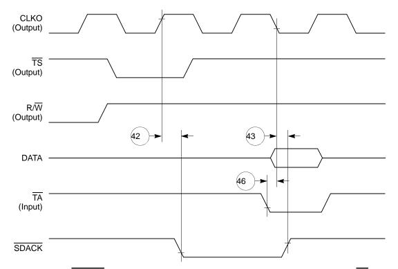
Figure 45. SDACK Timing Diagram—Peripheral Write, Externally-Generated TA
